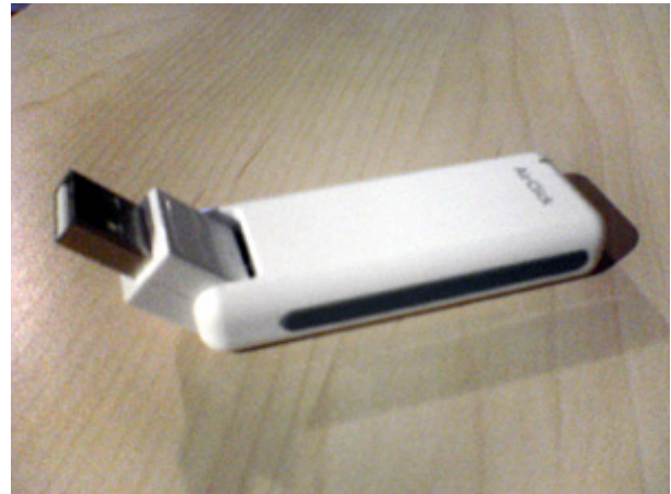
The AirClick USB receiver lives in any available USB port. A small USB extension cable comes with the receiver for use when the receiver cannot fit among other items around the USB ports.
