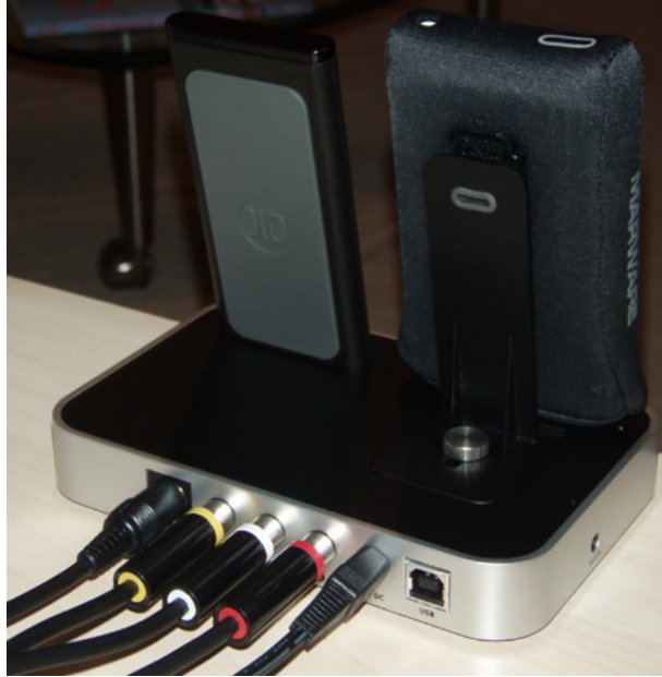
iPods are supported by an adjustable brace that slides forward and backward to accommodate various thicknesses of iPods and/or cases. The dock has standard RCA outputs instead of the single 3.5mm plug on Apple's dock. There's also an S-Video output and a standard B-type USB jack for connecting the dock to your computer.
