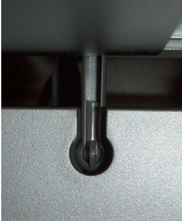
One of the ArtixScan M1's plastic hinges.
