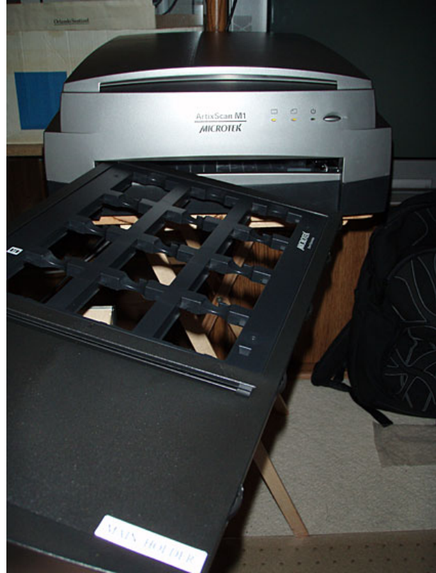
Because the transparency adapter is inserted directly into the scanner’s innards, dust can easily fly into the slot, or be carried from the adapter, into the scanner.
