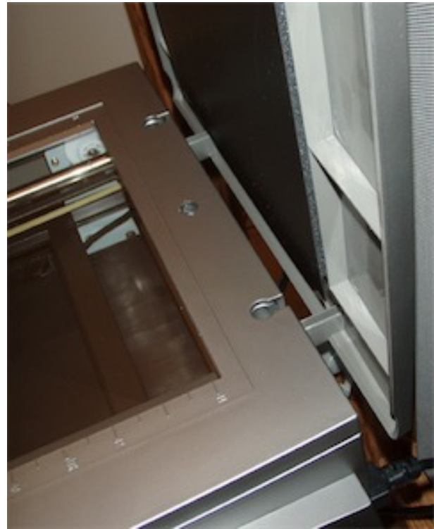
Even though the ArtixScan M1's cover is lightweight and thin, its support hinges seem extremely chintzy.
