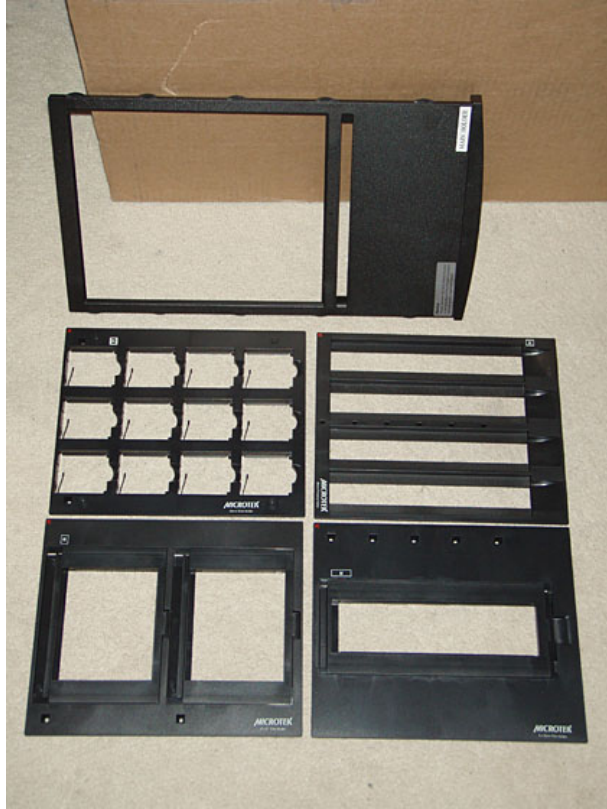
The ArtixScan M1's transparency adapters. The holder tray is above. The four adapters, clockwise from upper left: 35mm slides, 35mm filmstrips (negatives and unmounted slides), 6cm transparencies up to 22cm in width, and 4x5 medium format film.
