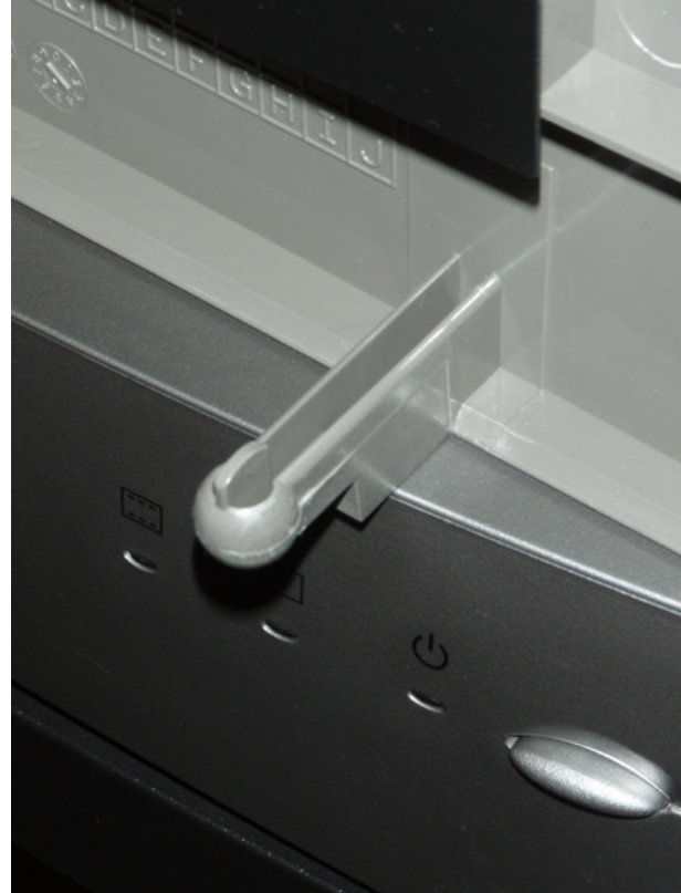
The scanner lid is removable. This image shows the entire strut that fits into the indentations on the scanner.
