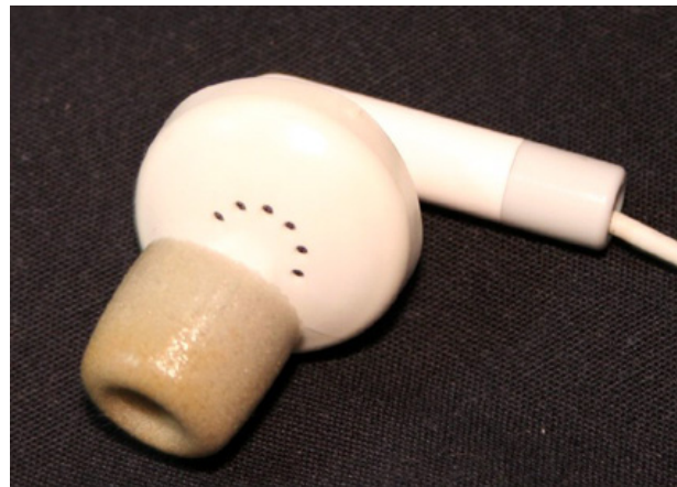
You can see a small nub at about the one o'clock position that causes discomfort after wearing the "enhanced" earbuds for awhile.
