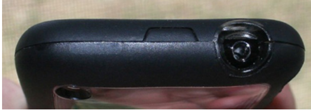
The headphone jack cutout is amply sized for even the largest headphone plugs.
