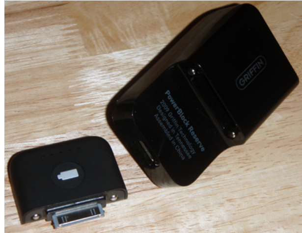
The Griffin PowerBlock accommodates the Reserve battery via a magnetic connection without the need of the dock connector, as well as a USB jack for directly charging an iPod or iPhone. The 2-prong power socket plugs fold into the PowerBlock for easier storage.
