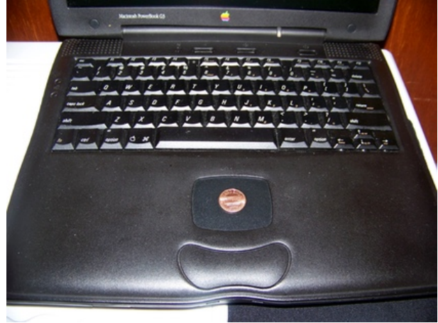
Compared to the trackpads found on 2009 MacBooks, the PowerBook G3's trackpad is tiny.
