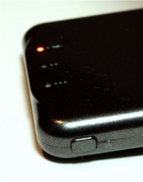
This small button, on the left side if you're looking at the open P-Flip, triggers a charge level test like the buttons on Apple's notebook batteries.
