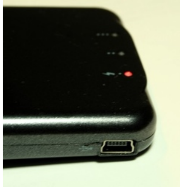
The right side of the P-Flip has its mini-USB port, through which you can charge your iPhone, sync it, or simply charge the P-Flip, or any combination of the three.
