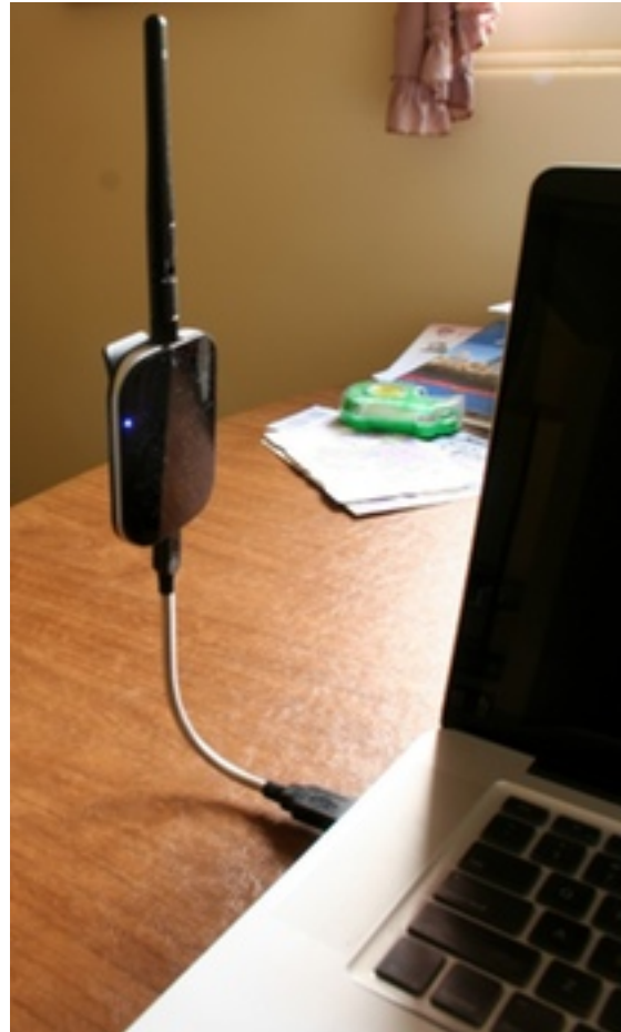
You can use the BearExtender's gooseneck USB cable and let it stick out the side of your laptop...
