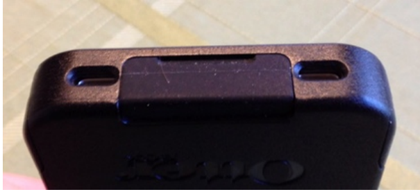
The silicone dust flap does a great job of keeping gunk out of the Dock connector.
