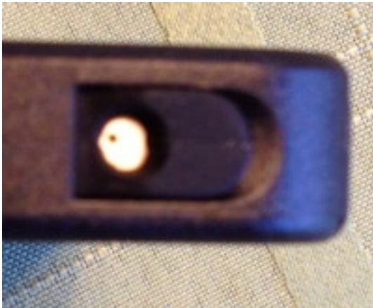
With the flap flipped up, the Commuter has more room for a large headphone plug than the Reflex does. The hole is for the noise-cancelling microphone.
