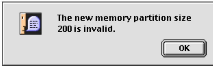
Alert Box for Situations Where Desired Memory Size Is Less Than the Application's Minimum Memory Size
