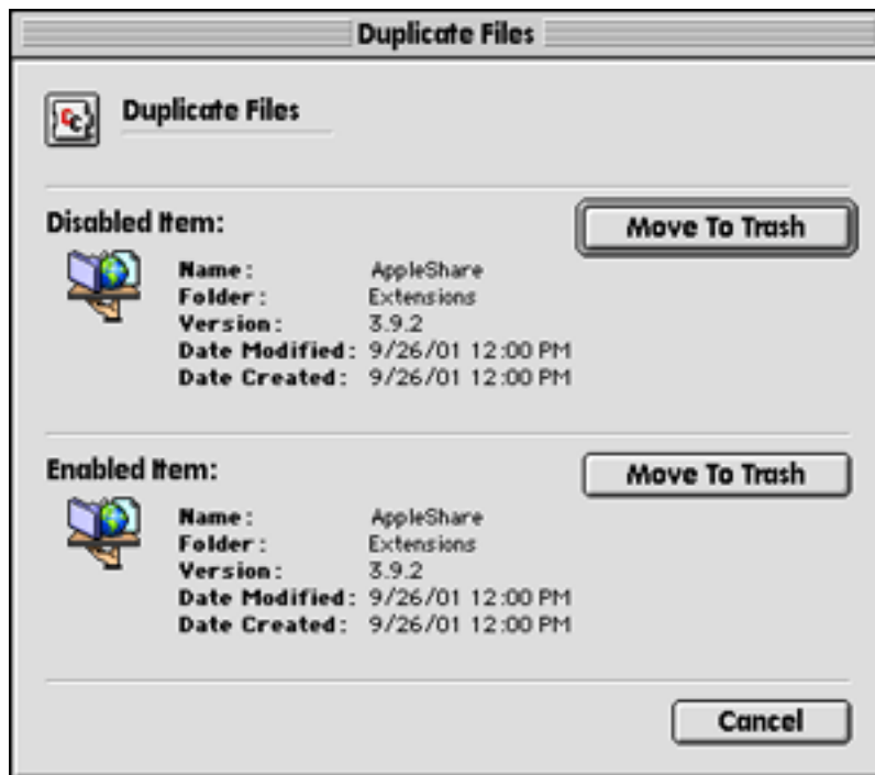
Figure 6: Conflict Catcher has detected two copies of the same extension after restarting back into the "Standard" set. In this case, both items are exactly the same and carry the same version number, but if one of them was older it could be trashed before ever making it into the startup process. Way to go, CC!
