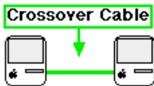
Two-Computer Crossover Connection
